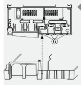
▶ Cut the left and right plastic flaps ® using an appropriate tool (e.g. knife) and carefully remove them from the case.
