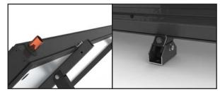
Position collector face up on the Support Strut, insert clips into Support Strut, and secure collector to Support Strut with clips. SunEarth recommends placing the Support Strut approximately  $10 \sim 20\%$  in from each end of the collector for maximum strength.
