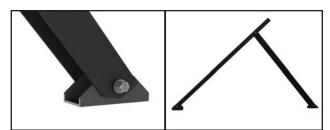
Assemble Rear Legs (2) (4) and (6)] and position the legs to the desired angle using the pre-drilled holes (See Angle and Spacing Table below). Mark the position of Rear Feet and securely fasten to mounting surface. Detach the Rear Leg from the Support Strut and Rear Feet. Lower the Support Strut to the mounting surface.
