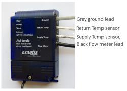
Joule can take 9-24V DC or AC. The terminals are polarity insensitive. Joule is shipped pre-wired.
