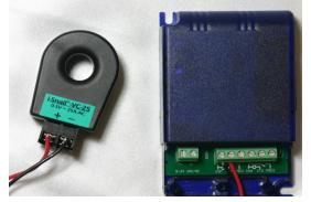
**Run** the live connection to the pump (black or red) through the hole in the CT. While some CTs are directional, that is not the case with this device.
